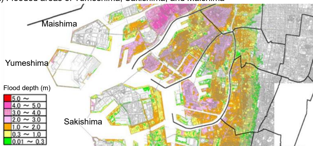
Figure 5. Flooding prediction in the major Nankai Trough Earthquake 6
