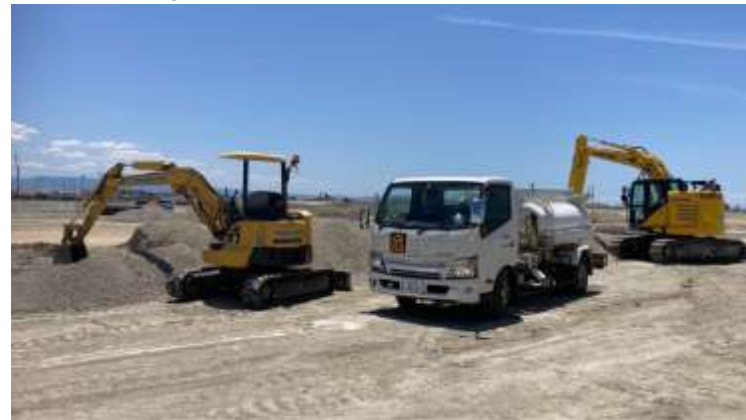
Construction machinery using the B100 fuel for the venue preparation work of the Osaka-Kansai Expo
