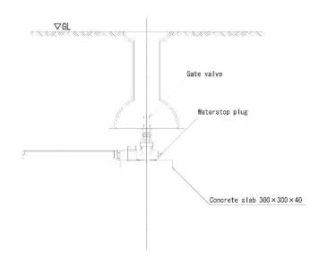
(1) Details of stopcock box + gate valve (30-50 A)  $\,$  S : NON
