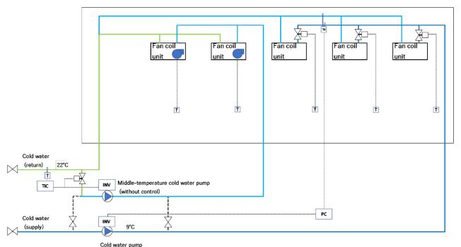
Figure 4.8 Overview of fan coil unit method system
